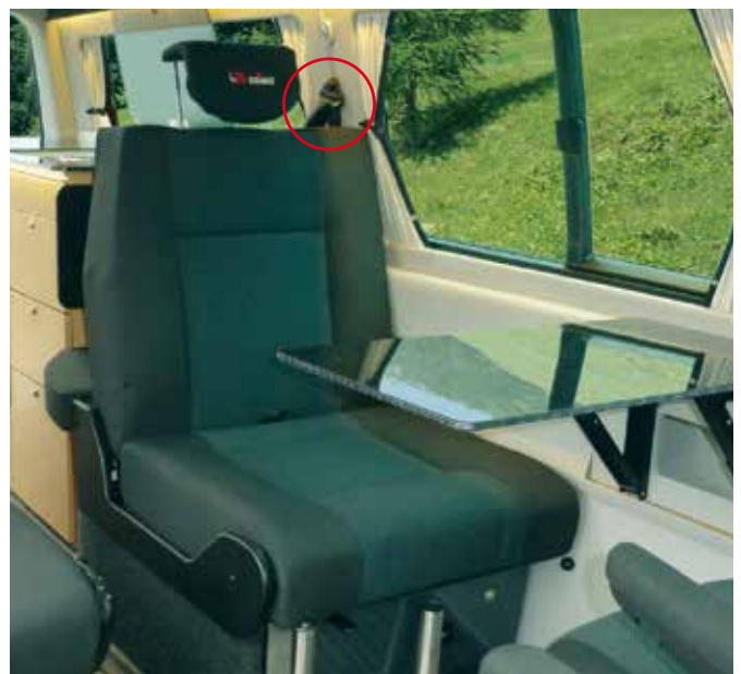
Fastening the belt to the vehicle spar
