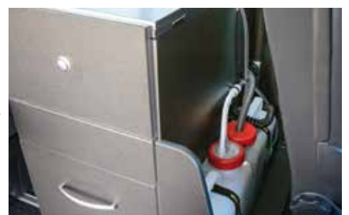
Integrated fresh and waste water canisters
