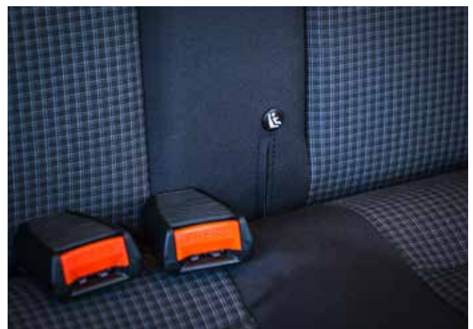
Seat with fabric cover Double Grid T6.1. and Isofix attachment point
