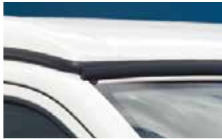
The sleeper roof super flat short wheelbase is supplied with a rubber spoiler as standard.
